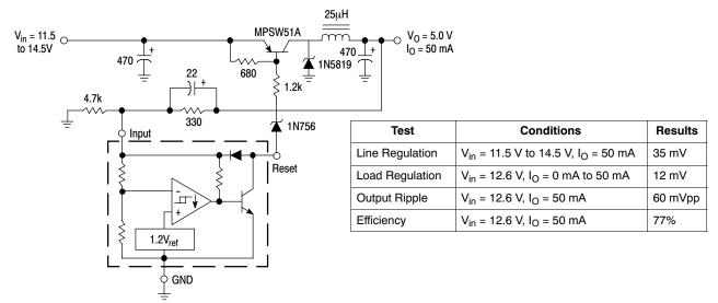
Figure 13. Low Power Switching Regulator
