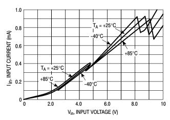
Figure 5. Input Current versus Input Voltage
