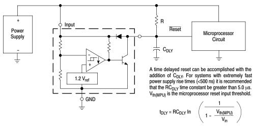
Figure 9. Low Voltage Microprocessor Reset
