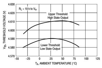
Figure 4. Comparator Threshold Voltage versus Temperature
