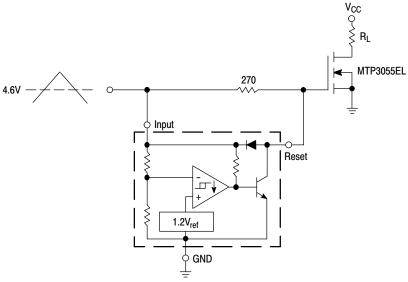
Overheating of the logic level power MOSFET due to insufficient gate voltage can be prevented with the above circuit. When the input signal is below the 4.6 V threshold of the MC34064, its output grounds the gate of the  $L^2$  MOSFET.
