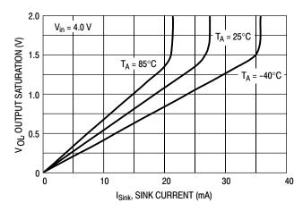
Figure 6. Reset Output Saturation versus Sink Current
