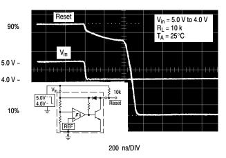
Figure 7. Reset Delay Time
